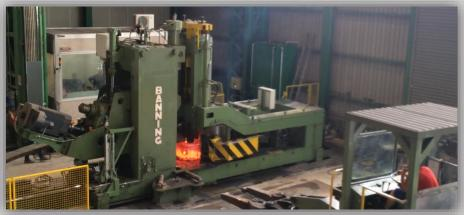
1 rolling mill WAGNER 100/80 for radial-axial rings: maximum diameter 2500mm x max. height 650 mm. 1 rolling mill WAGNER 80/50 for radial-axial rings: maximum diameter 2000mm x max. height 400 mm.
